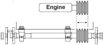
Figure 48. Pulley Alignment
